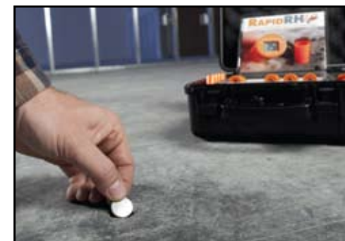
Place metal disk over Smart Sensor before encapsulating
